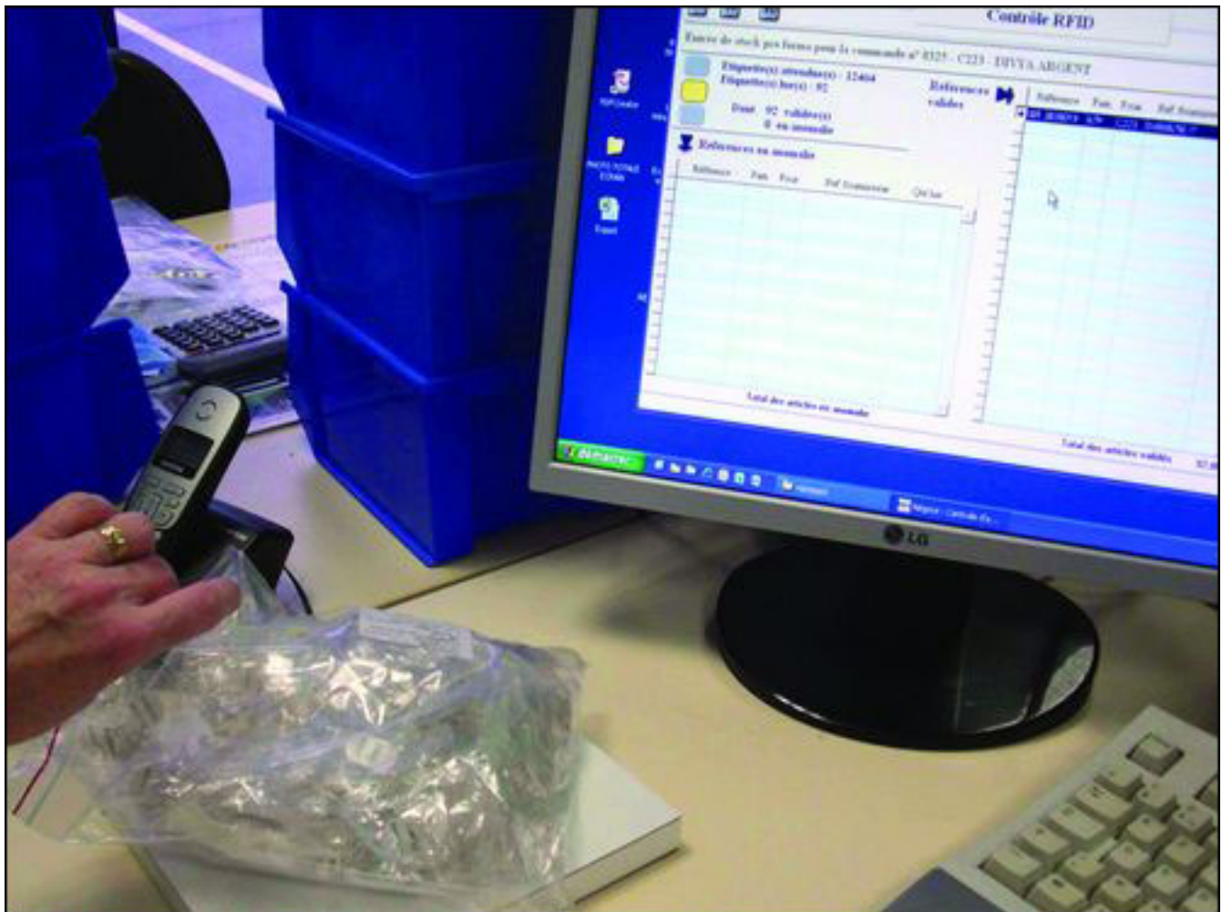
Staff members at Cleor's DC place a bag of ordered items on an RFID mat, in order to verify a shipment's accuracy and update its status.
