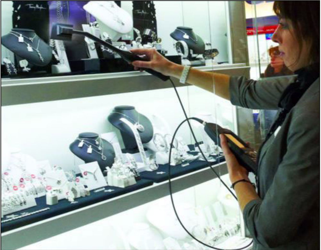
To take inventory of items in a store's display cases, Cleor's staff uses a handheld RFID reader, holding a paddle antenna over each item to read its tag.
